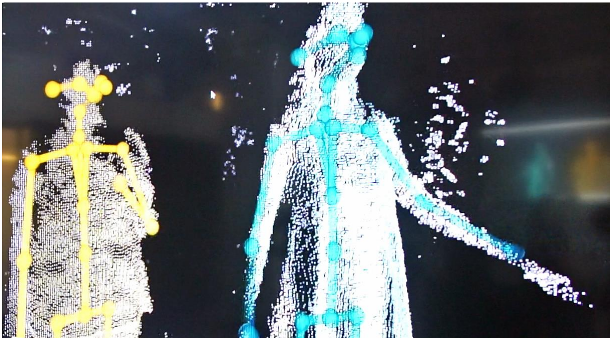
Figure 3. Pedestrian identification, motion detection, and pose inference using RGB + D depth mapping.
