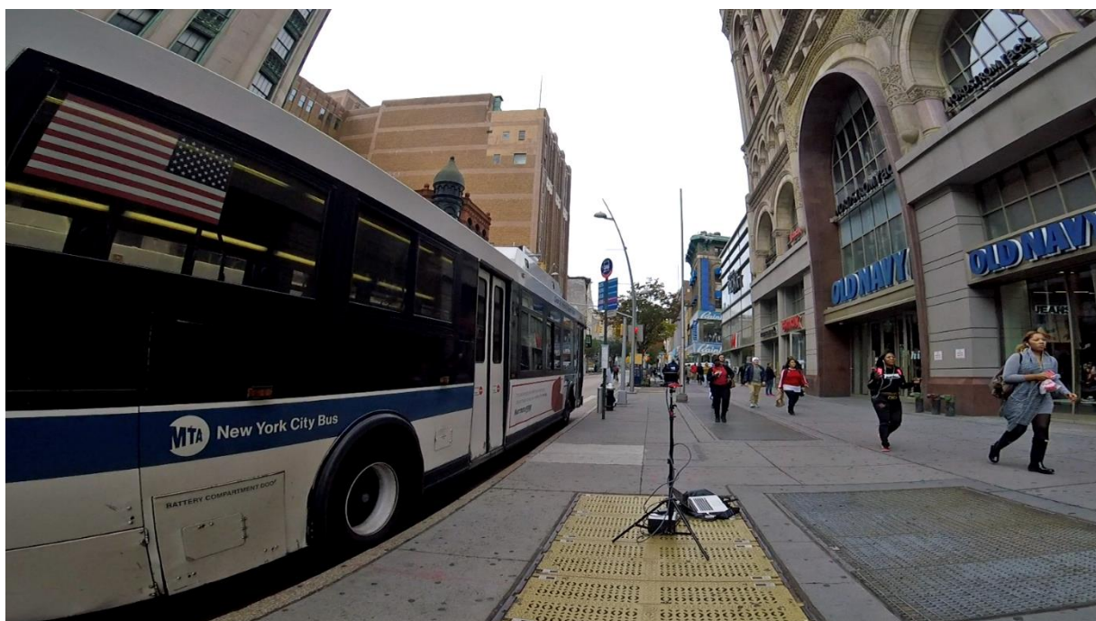
Figure 4. Automated analysis of pedestrian footfall on a retail high street with a LiDAR sensor positioned in the midst of high street dynamics.
